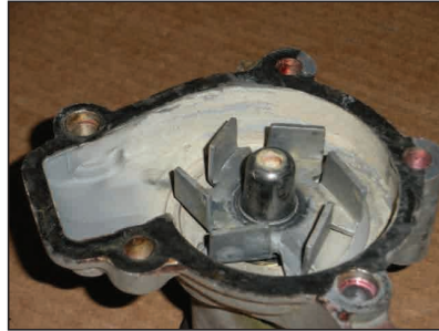
Deposits / Calcium Buildup
