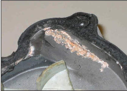
Deposits / Calcium Buildup
